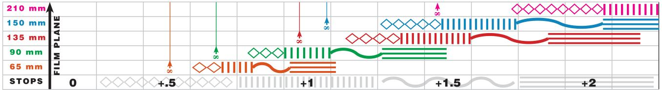
Align with the cameras film plane and read the exposure correction value from the scale at the nodal point of the lens. • Bellows Extension and Exposure Compensation Guide From www.cookseytalbottgallery.com © 2007 All Rights Reserved.
